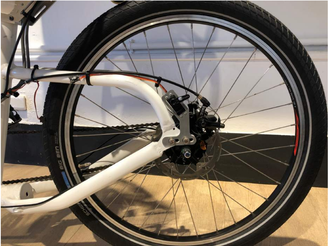
Figure 3-3: High torque motor to control bike brake.
