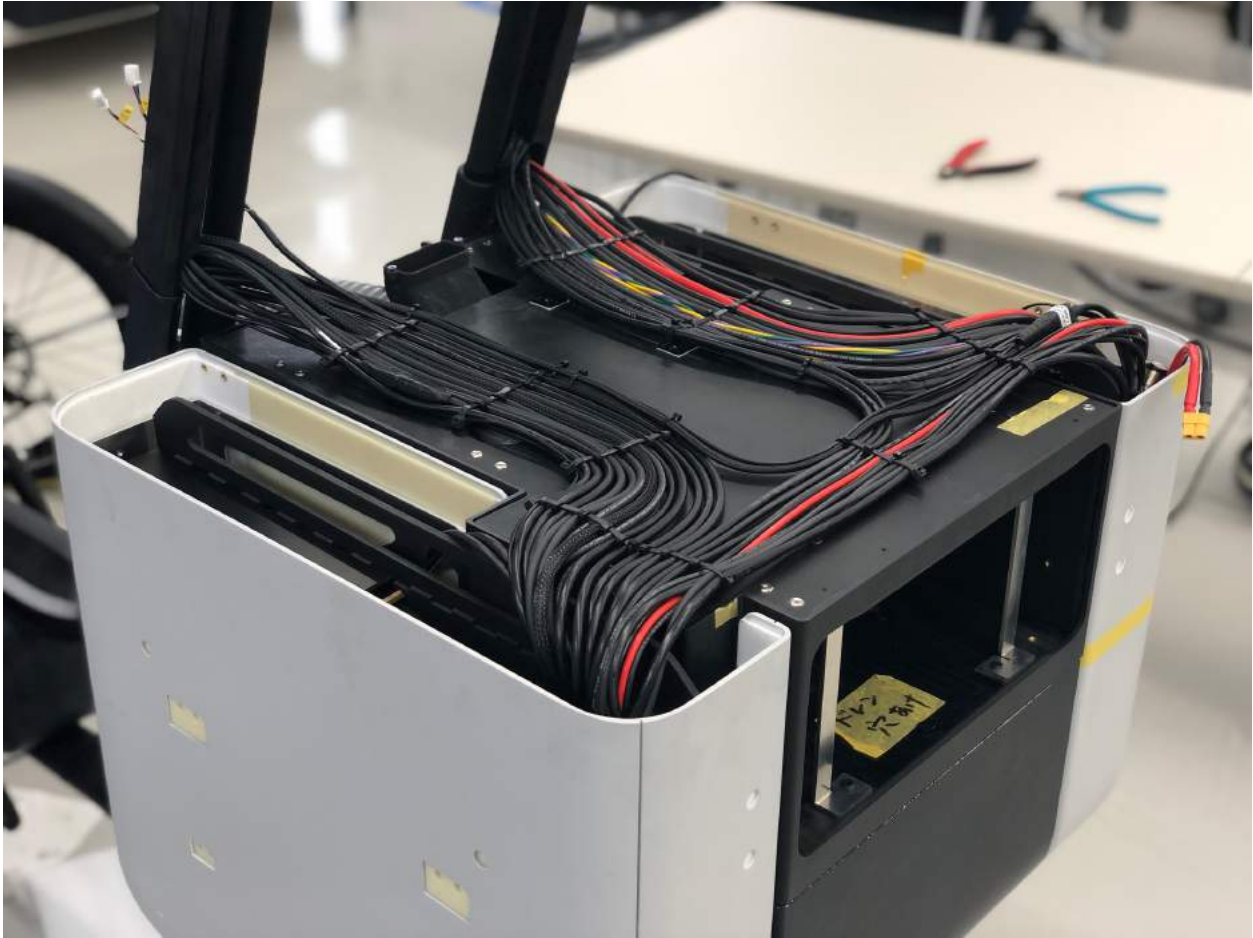
Figure 3-16: The IDK+ installed in the rear part of the PEV.
