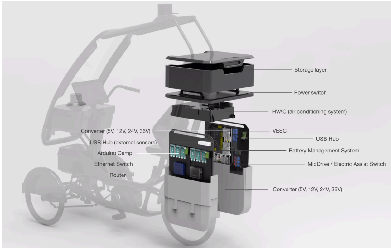
Figure 3-14: The IDK+ and latest PEV integration.
