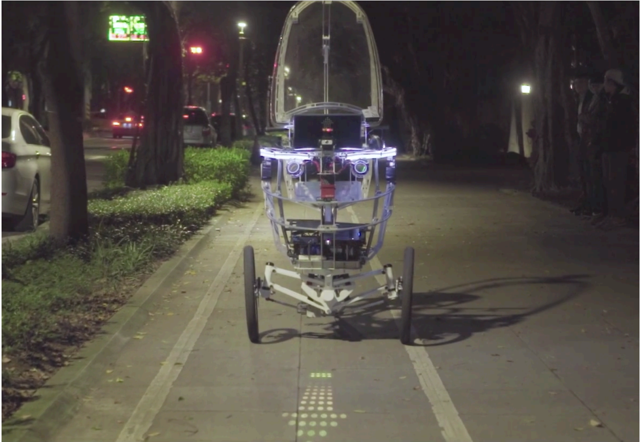
Figure 4-10: Projection showing the intention of the PEV.
