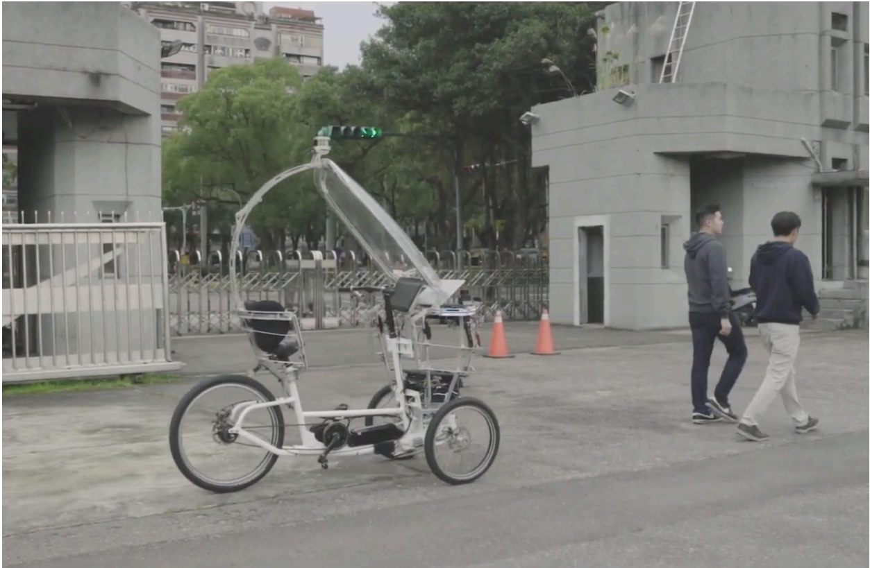
Figure 4-15: PEV following mode: PEV follows a rider using IDK Standard system.
