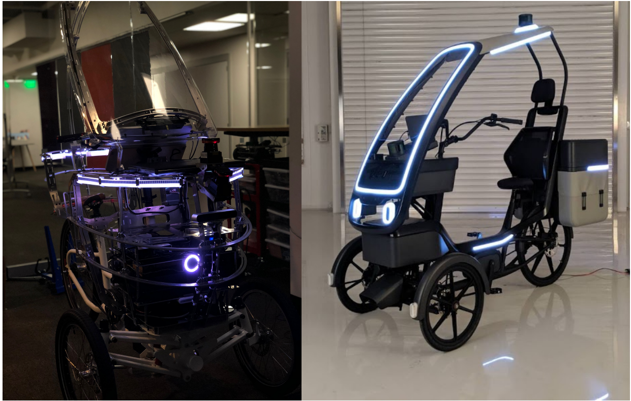
Figure 4-6: Lighting design built by IDK Lite (left) and IDK+ (right)
