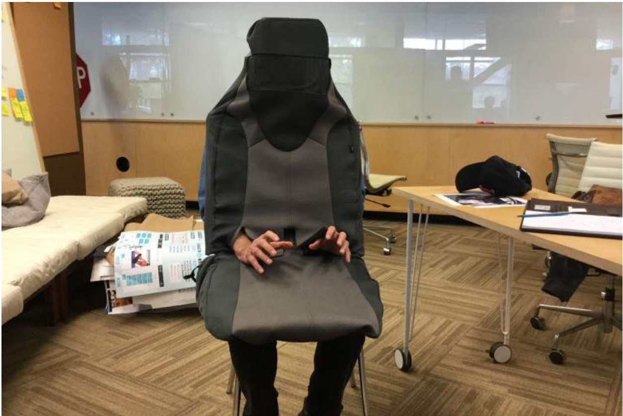
Figure 2-4: Example of Wizard of Oz experiment to disguise the driver [24].
