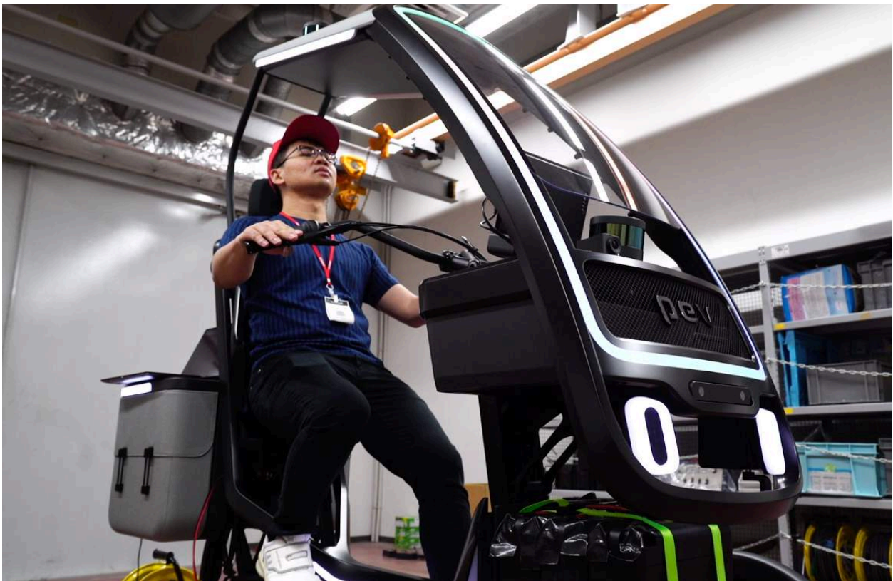
Figure 4-16: A rider testing rider state monitor (RSM) in the PEV
